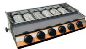
MVDK-736 GAS Gas Type:LPG Gas pressure:2800pa Size:800×400×180mm Burn Value:22.5Mj
