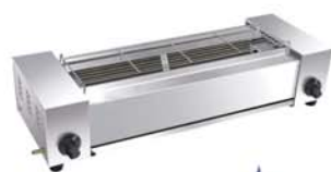
MVSJ-702 GAS Gas Type:LPG Gas pressure:2800pa Size:1070×400×250mm Burn Value:35Mj
