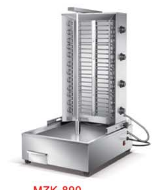
MZK-890 Electric Shawarma Machihe (3-element) Size:500×650×900mm Heat Power:6KW Motor Voltage:220V/380V Motor Speed:4.8r/min Temperature:50~300℃
